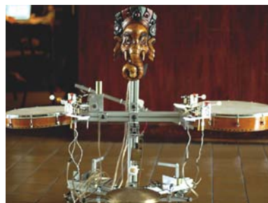
The GANAPATIBOT succeeded the MahaDeviBot (page 36) and includes more options for striking the percussion instruments, along with speakers that play sounds from an iPod mini.
