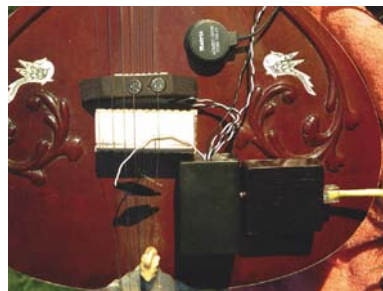
THE ELECTRONIC SITAR (ESitar) combines the sitar with software that enables a performer to connect to a laptop and interact with robotic instruments.
