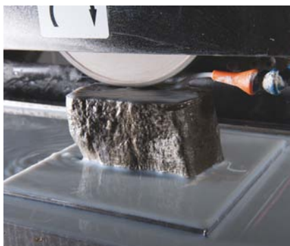
Malooof’s diamond-studded grinding wheel at work.
